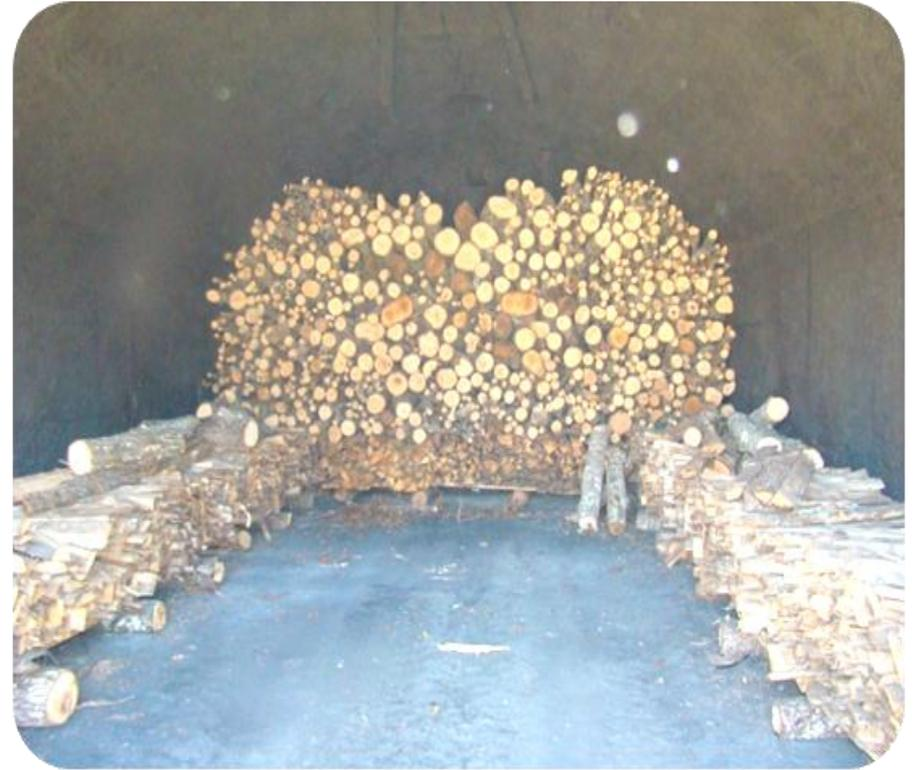
**This is the inside of the kiln where the wood is hand stacked very carefully up to the top of the roof. The ceiling line is 14 feet tall. When the burning is over the stack remains 7 feet tall.**
