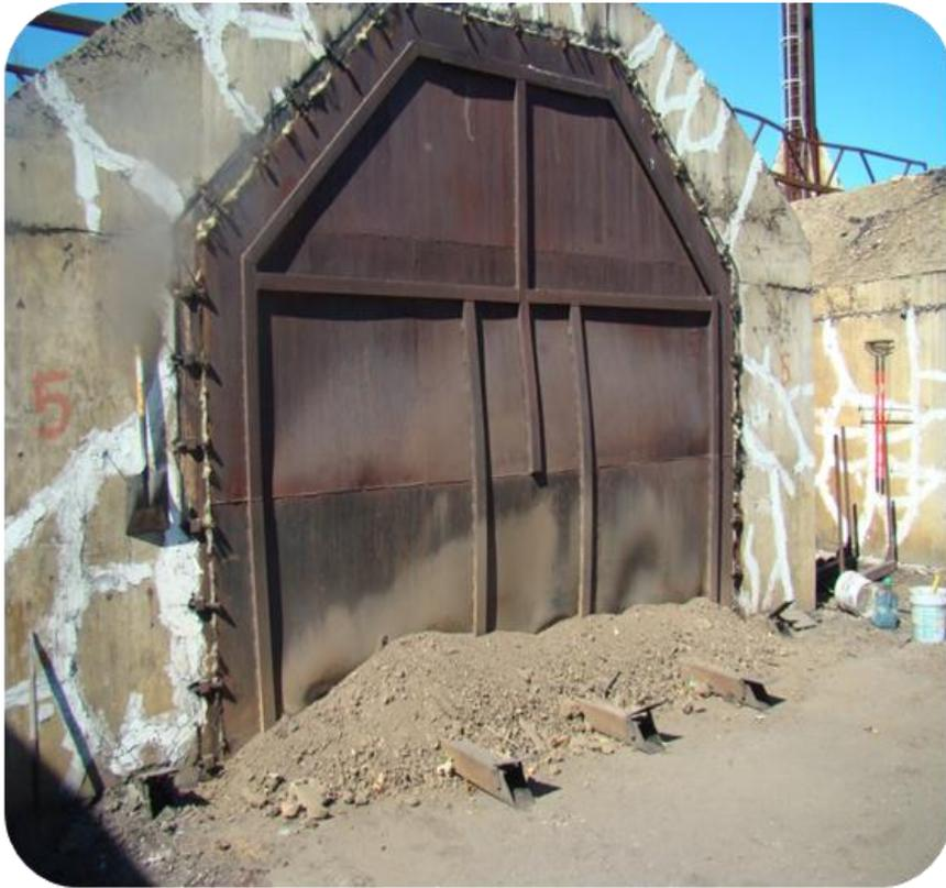
**This is the outside of the kiln with the door tightly sealed, even up to the point of hand stuffing fiberglass insulation by hand in any small cracks that may be exposed. Also notice that the kiln has white patch lines on the concrete. This patchwork is done daily to prevent any smoke from escaping into the atmosphere.**
