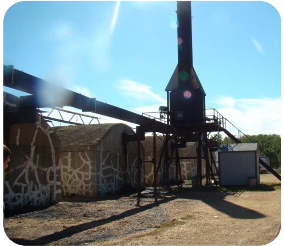
**This is the afterburner which services a complete line of 6 kilns. This afterburner burns the smoke from the kilns at 2000 degrees. With this afterburner, the emissions that are released into the atmosphere are 99.99763 % smoke free.**
