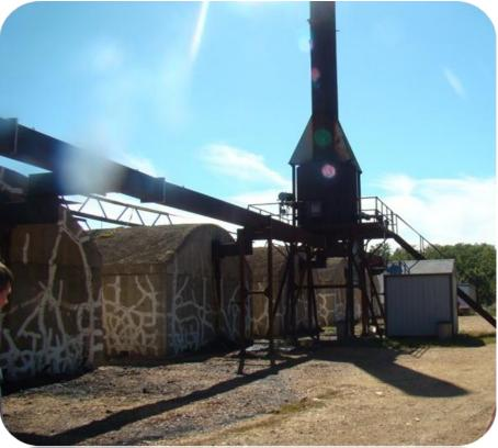
This is the outside of the kiln with the door tightly sealed, even up to the point of hand stuffing fiberglass insulation by hand in any small cracks that may be exposed. Also notice that the kiln has white patch lines on the concrete. This patchwork is done daily to prevent any smoke from escaping into the atmosphere.
